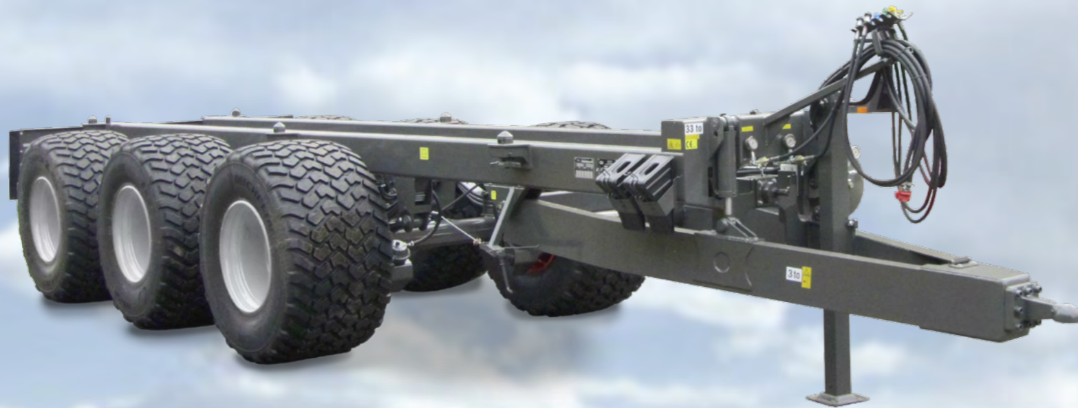
Tridem running gear with PTO shaft drive for the drives of the body.
