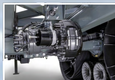
The drive is by oil motor and cardan shaft. Disc brakes provide deceleration.
