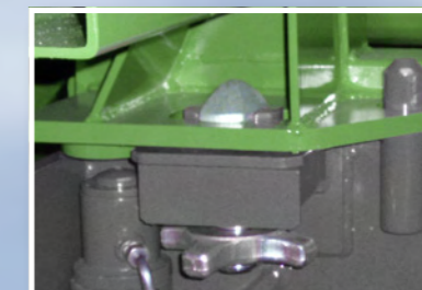
The HAWE rectangular system with Twist-Lock locking (rectangular tubular frame) has a very low gravity point and lays the foundation for flexible transportation of agricultural products using different bodies. All drives for HAWE bodies are built into the body on option. This reduces the changeover time and prevents faults. The drive shafts and hydraulic hoses are connected by means of quick-release couplings – simple and safe.
