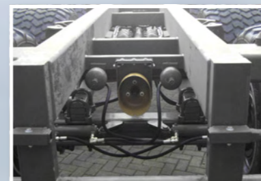
Tridem running gear with PTO shaft drive for the drives of the body.
