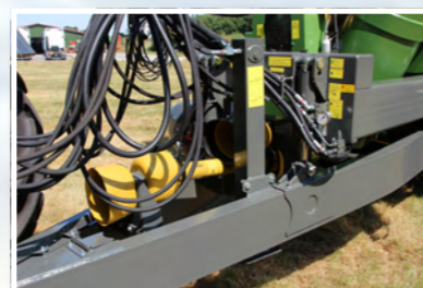
Hydraulic parking stand and hydraulic drawbar suspension.
