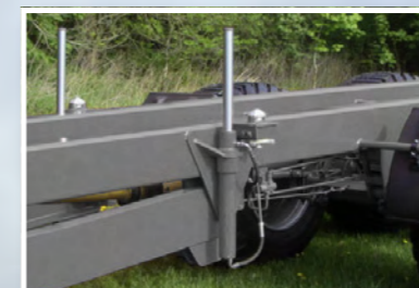
Lifting rams to remove and install the different bodies.
