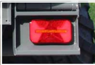
Pendulum suspended **LED taillights**. (protective grille available as an accessory).
