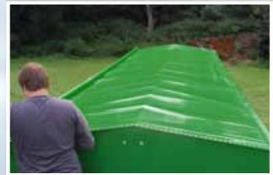
The HAWE **roll-up cover system** is very easy to use. The cover is firmly attached by a toothed rack system; additional ratchet fixings or similar are unnecessary. It is operated from a platform which is supplied as standard equipment and is accessed by a folding ladder.
