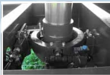
**Shut-off valve** and **rapid lowering valve** on the tipping ram.
