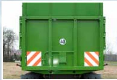
Reinforced **tailgate** with a solid frame made of square tubing for permanent sealing.
