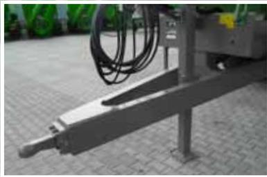
Hydraulic parking stand and mechanical **drawbar suspension**.
