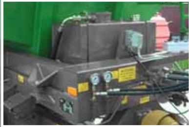
Oil supply via **on-board hydraulics** with electro-hydraulic control.
