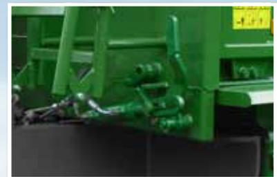
The **sidewall unlocking system** can also be hydraulically actuated as an option.
