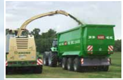
HAWE CSW 5000 with tridem running gear and parabolic suspension with self-steering for the first and third axle. Positive steering is available as an option.
