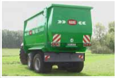
HAWE CSW 4000 with tandem running gear and hydraulic suspension, incl. lift axle and self-steering.
