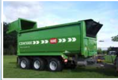
HAWE CSW 5000 with tridem running gear and parabolic suspension with self-steering for the first and third axle. Positive steering is available as an option.
