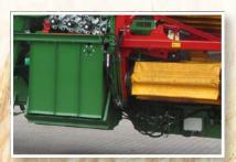
The **collection bunker** for trash and soil offers up to approx. 3 cubic metres volume. The bunker is emptied back in the field hydraulically via two discharge flaps.
