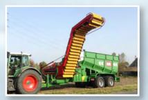
The transfer height is approx 4.1 m. the folding of the elevator belt allows a particularly gentle transfer into the receiving vehicle. The KUW is also suitable for other crops such as Carrots, Onions, Beetroot, Parsnips etc.
