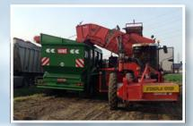
The mounted steel container is equipped with a **rolling floor** with stable conveyor chain and galvanized steel strips. The cross elevator is 1200 mm wide and allows a discharge capacity of up to 120 t/h.
