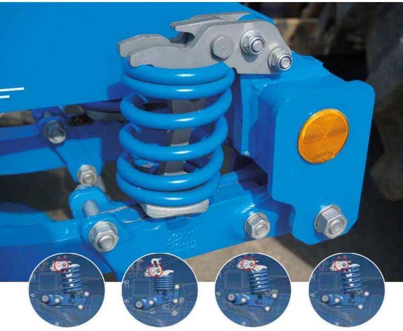
When hitting obstacles, the concave discs deflect independently upwards and rapidly return to their working position. In the basic position, the coil spring pushes the stop upwards.
